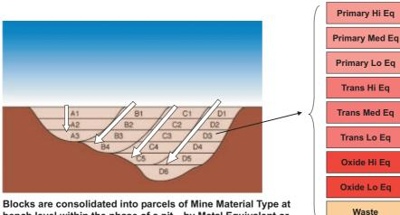
Blocks are consolidated into parcels of Mine Material Type at bench level within the phase of a pit – by Metal Equivalent or Equivalent Value
