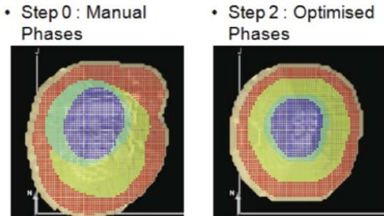
Figure 3. Comparison between manual and optimized pit phases
