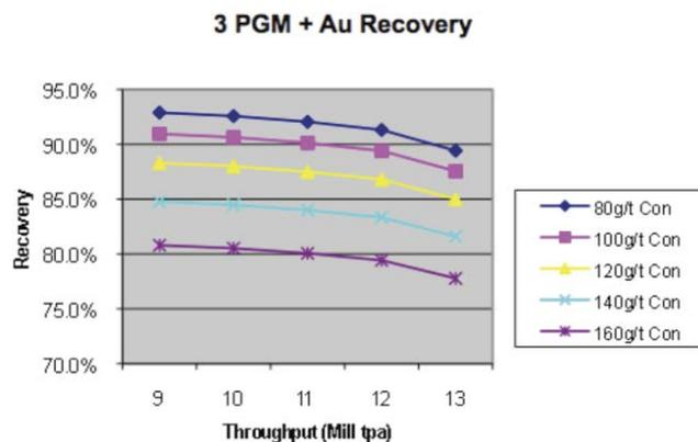
Figure 11. Effect of downstream processing constraints on concentrate grade
