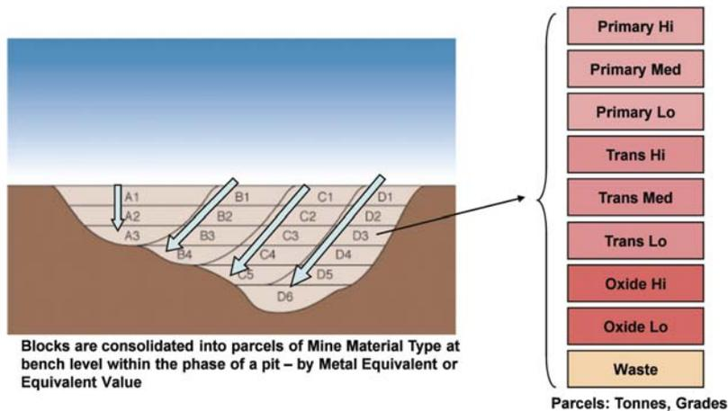
Figure 5. Grade banding for maximum throughput in multi-element systems
