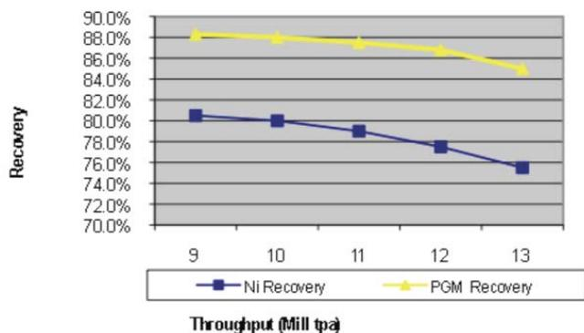
Figure 10. Potential to optimize plant by varying throughput and recovery
