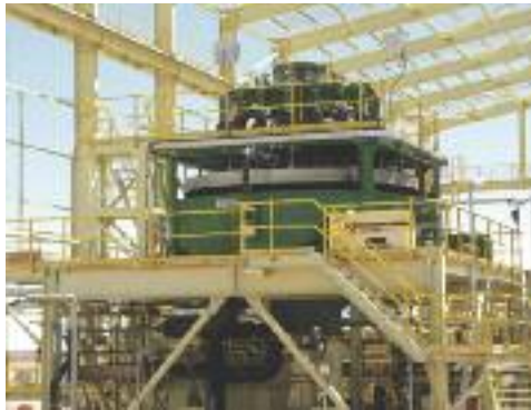
The Jameson flotation cell, developed by Graeme Jameson, who is inducted in the Concentration category
