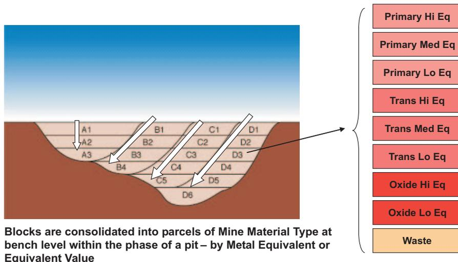
**Blocks are consolidated into parcels of Mine Material Type at bench level within the phase of a pit – by Metal Equivalent or Equivalent Value**
